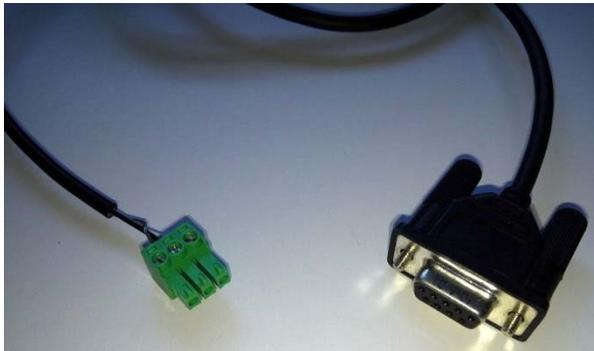
most commonly seen on desktop PCs or controllers, also known as "serial port". The pin numbers are usually molded on the connector. You only need to connect 3 of the 9 wires of the D-sub connector:
